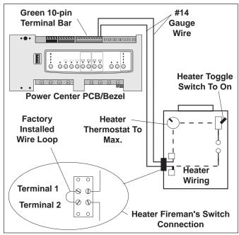
Figure 9. Lite2 Heater Connection
